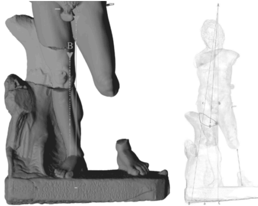
Figure : Restorer calculation as rigid solids, gravity vectors of blocks and those of their stacks
